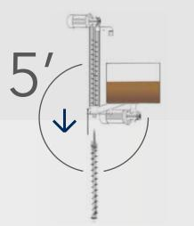
Technical data Electrical specification: 400 V three phase 50 Hz Power required: 1 Kw - 16 A - 5 poles Tank capacity: 12 Kg Hourly production rate: 55 Kg Cooling unit: 900 frigorie/h Dimensions: h. 1470 mm, w. 380 mm, d. 740 mm inclusive of vibrating table: w. 670 mm
